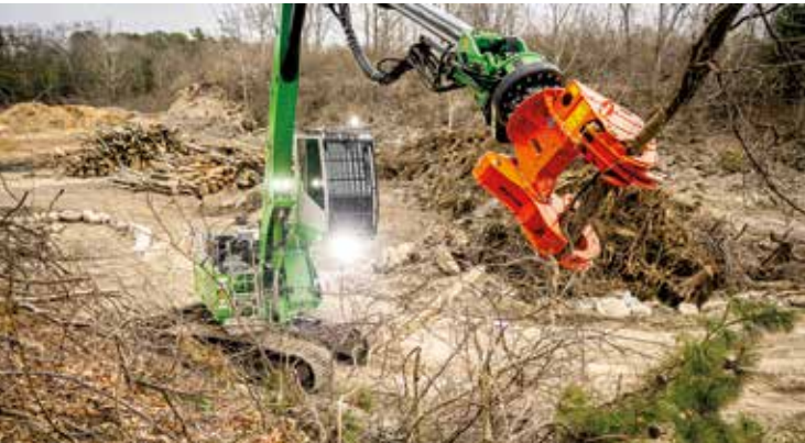
Woodcracker® C300 on Sennebogen 718 crawler excavator - construction site clearing
