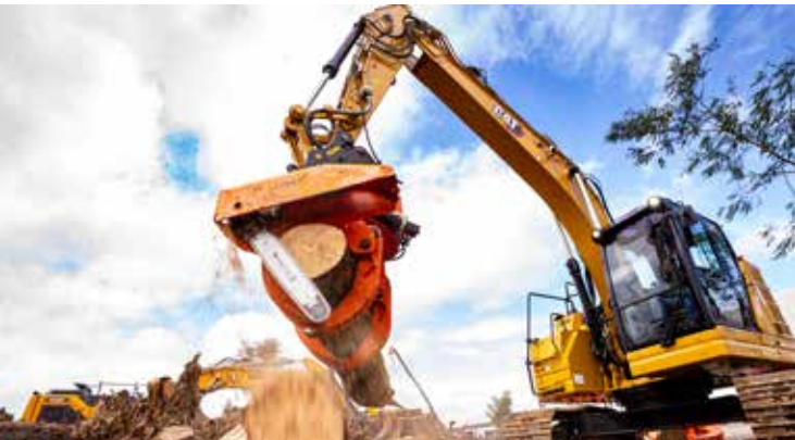
Woodcracker® CS800 dualGrip on CAT325 crawler excavator - high sawing performance
