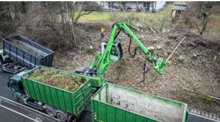
Woodcracker® C300 on Sennebogen 718 crawler excavator - roadside maintenance
