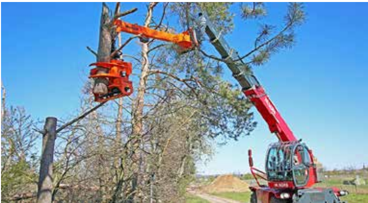
Woodcracker® CS620 crane with extension on a telehandler
