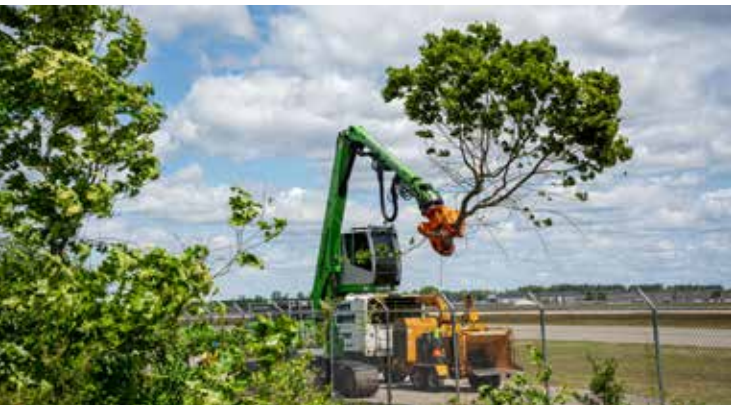
Woodcracker® C300 on Sennebogen 718 crawler excavator - safety tree felling
