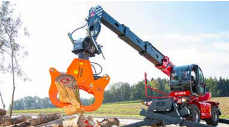
Woodcracker® W1000 on Magni telehandler - various mounting options
