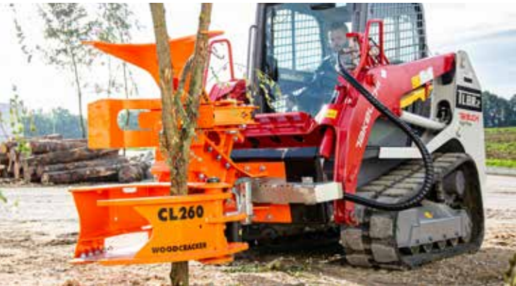
Woodcracker® CL260 on Takeuchi Skid Steer - cut - hold - drive
