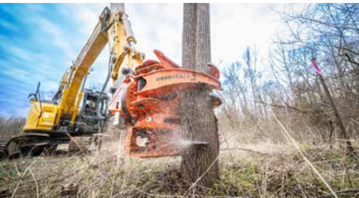
Woodcracker® CS545 compact on Kobelco SK140 crawler excavator - high sawing performance
