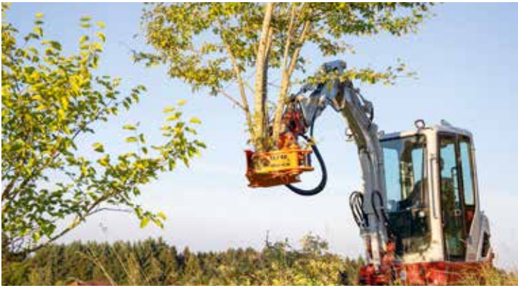
Woodcracker® CL140 on Takeuchi TB225 crawler excavator - removal of small trees and bushes
