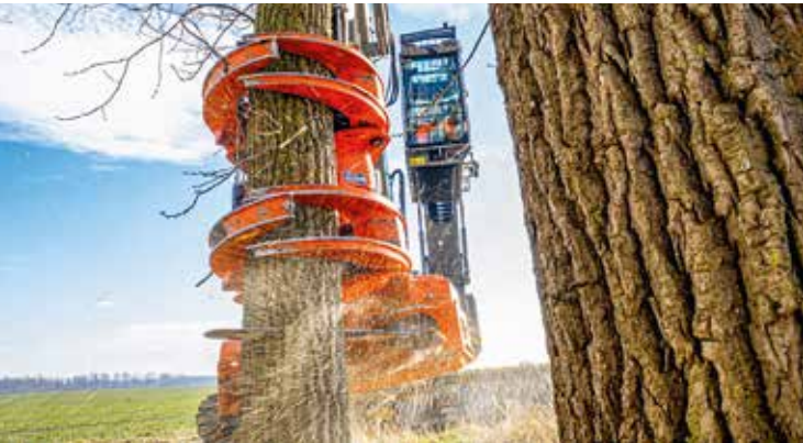
Woodcracker® CS800 dualGrip on Sennebogen 825 crawler excavator - the grapple adapts to the tree
