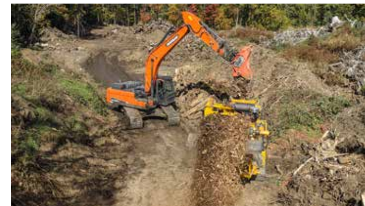
Woodcracker® R1300 on Doosan DX255 crawler excavator - chipping the rootstock for further processing
