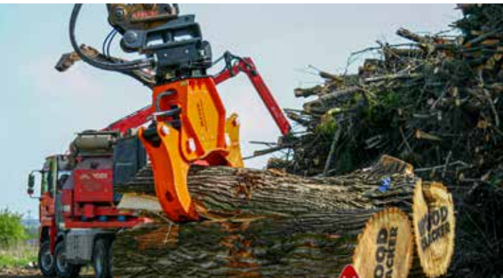
Woodcracker® W1350 on truck - pre-splitting wood for the chipper
