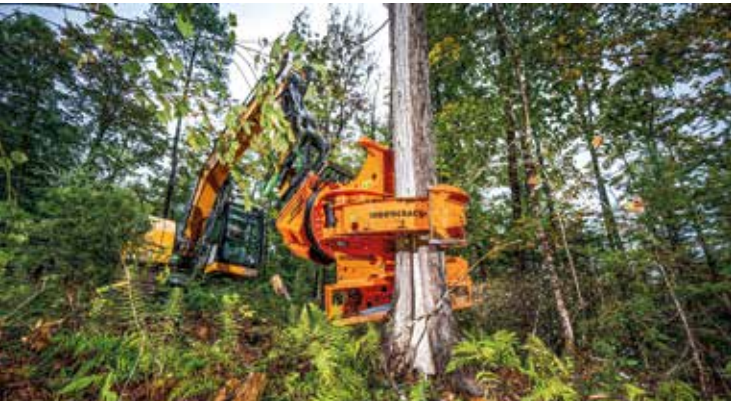
Woodcracker® CS610 on LH R914 crawler excavator - safe grip during the sawing process
