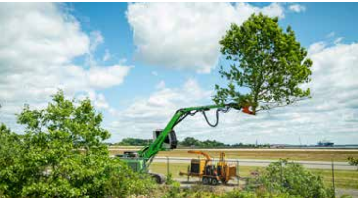
Woodcracker® C300 on Sennebogen 718 crawler excavator - land clearing
