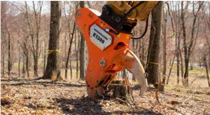
Woodcracker® R1300 on CAT330 crawler excavator - high splitting force
