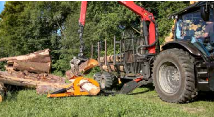
Woodcracker® L700 with stand unit on timber trailer - low effort for splitting
