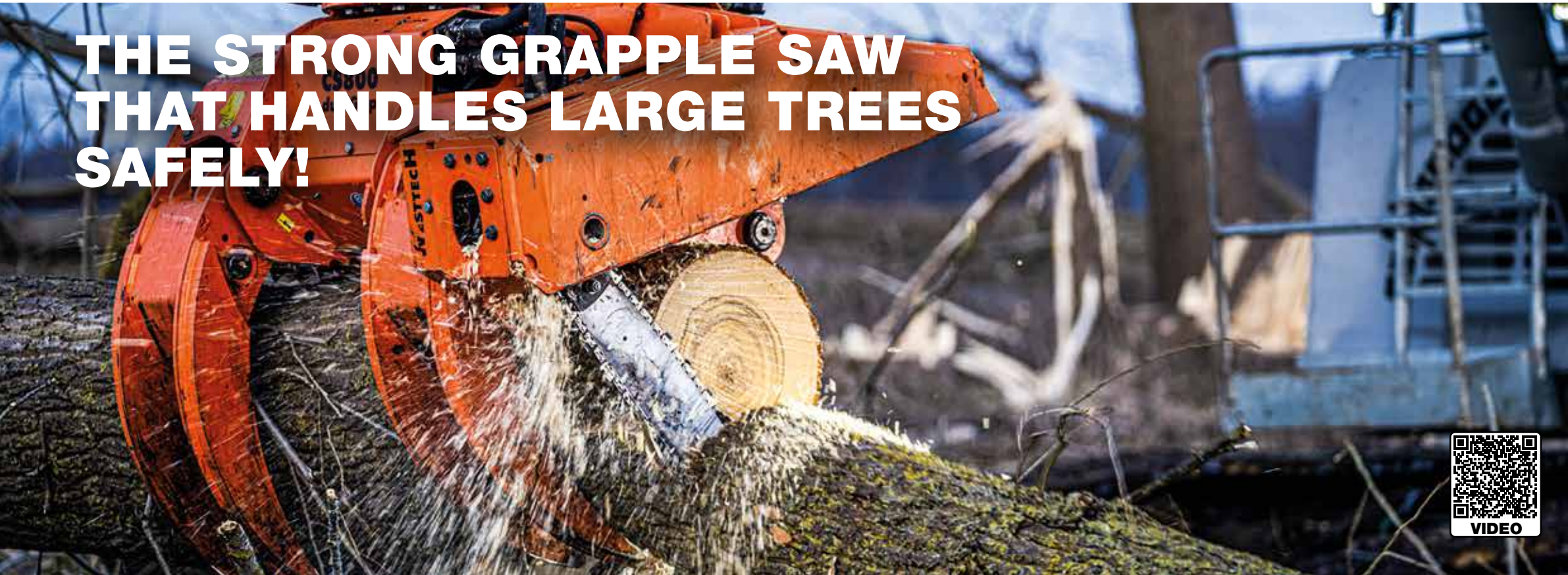
Woodcracker® CS800 dualGrip on Kobelco SK300 crawler excavator - the strong grippers hold the tree firmly
