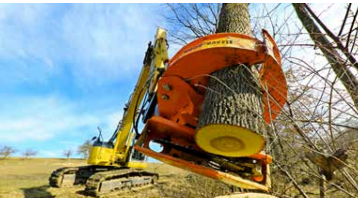
Woodcracker® CS610 compact on Komatsu 225 crawler excavator - high-diameter sawing
