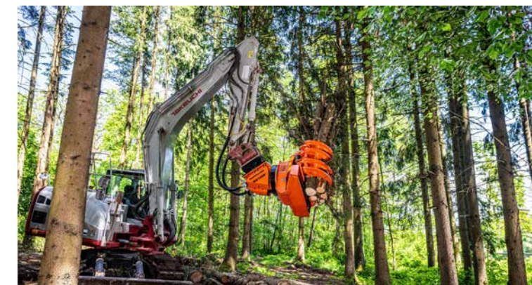
Woodcracker® WG1600 on Takeuchi TB2150 crawler excavator - optimal attachment angle for felling and processing
