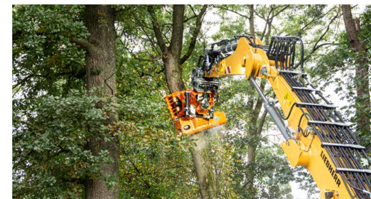
Woodcracker® WG1600 on Liebherr LH22 wheel excavator - tree felling
