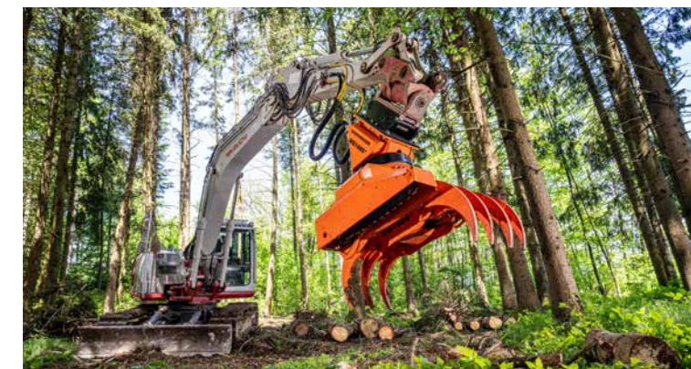
Woodcracker® WG1600 on Takeuchi TB2150 crawler excavator - enables fast material handling
