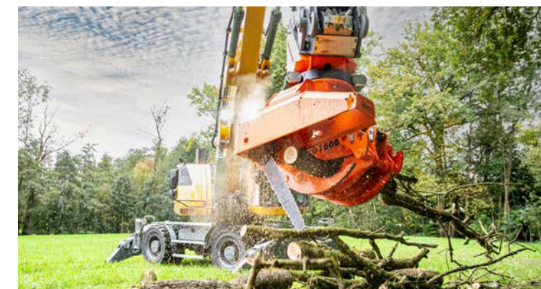
Woodcracker® WG1600 on Liebherr LH22 wheel excavator - high sawing performance
