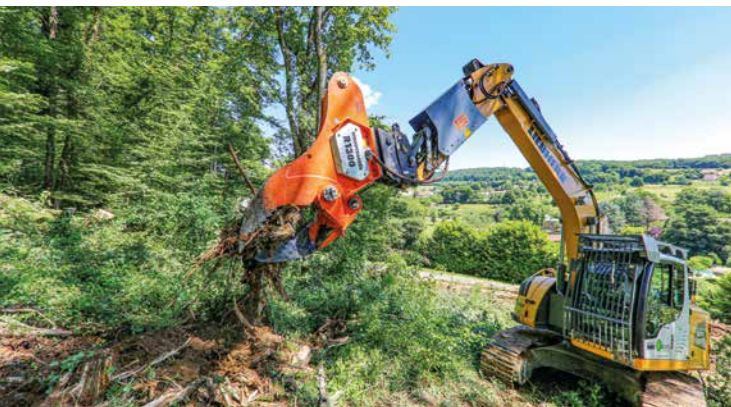
Woodcracker® R1300 on Liebherr R920 crawler excavator - careful removal of the entire rootstock from the ground
