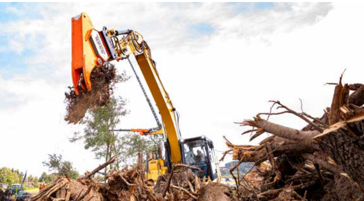
Woodcracker® R1300 on CAT325 crawler excavator - pre-chipping for the transport
