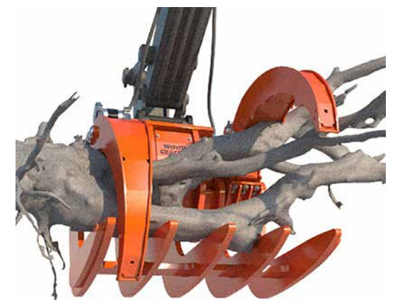
The gripper fingers adjust individually to the crop.
