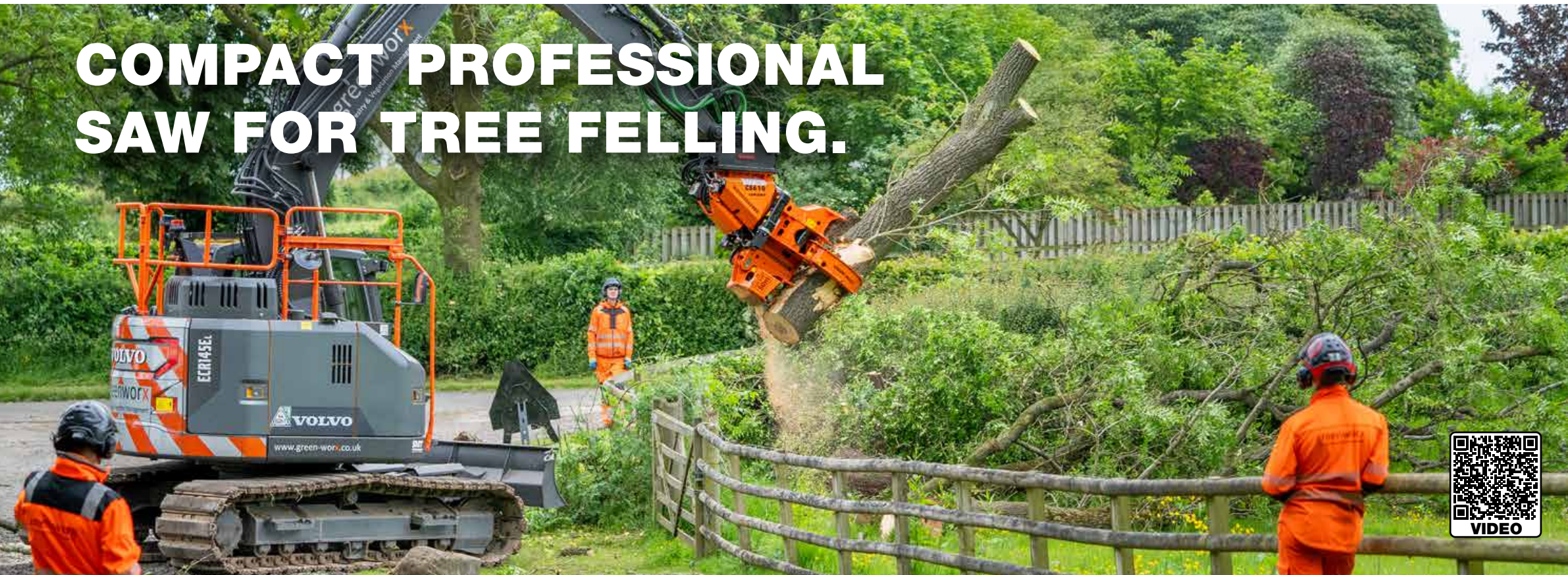
Woodcracker® CS610 compact on Komatsu 225 crawler excavator - high-diameter sawing
