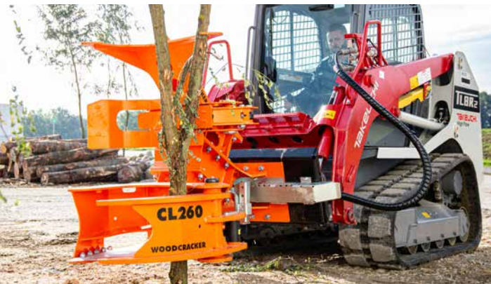
Woodcracker® CL260 on Takeuchi Skid Steer - cut - hold - drive
