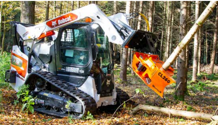
Woodcracker® CL260 on Bobcat Skid Steer - easy to handle in tight spaces
